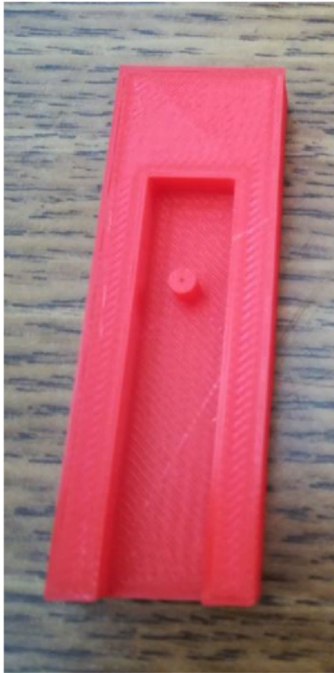
Figure 17. 3D printed valve test base
