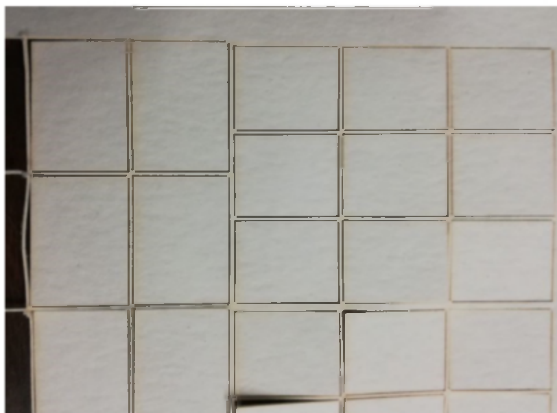
Figure 9. Laser cut blotting paper parts used in the final device
